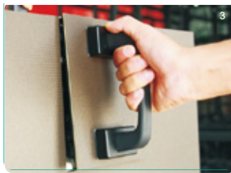
3. Pulling the magnet slowly, module will be apart from cabinet
